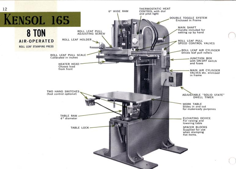
The new Kensol 165 eight ton, double toggle press is the most versatile hot stamper ever designed. This machine is similar to the Kensol 65 except for the frame design. The 165 will stamp items from flat to twenty inches high. Due to the extra deep 12 inch throat, the center of a 24 inch wide
