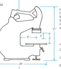
5 x 6 Inches . . . . . . 800 Watts 6 x 8 Inches . . . . . . 1,000 Watts 6 x 12 Inches . . . . . . . 1,500 Watts 9 x 12 Inches . . . . . . . 2,100 Watts HEAD STROKE: 3 Inches DEPTH OF THROAT: 9 Inches MAXIMUM OPENING: 5 Inches WILL HOT STAMP ITEMS UP TO 2 INCHES HIGH PRESSURE RANGE: UP TO 3 TONS WORK TABLE:
